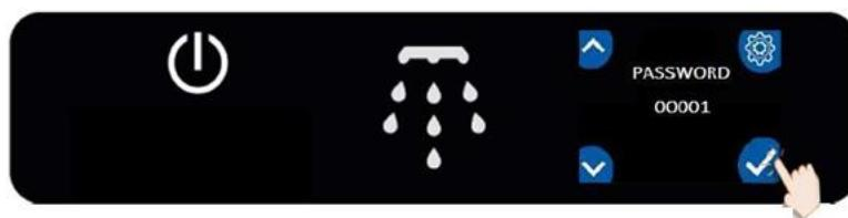
Enter the password "1" by using "up" and "down" buttons. Hold for 3 seconds to confirm
